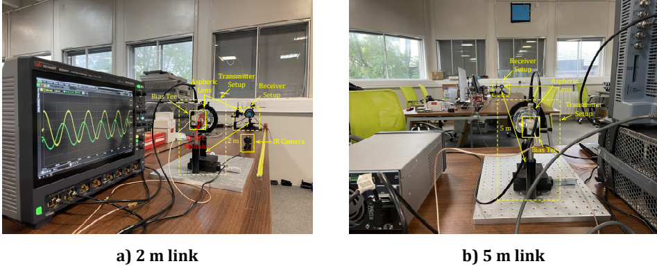
Fig. 2. Experimental setup for 2 m and 5 m OWC link configurations.
